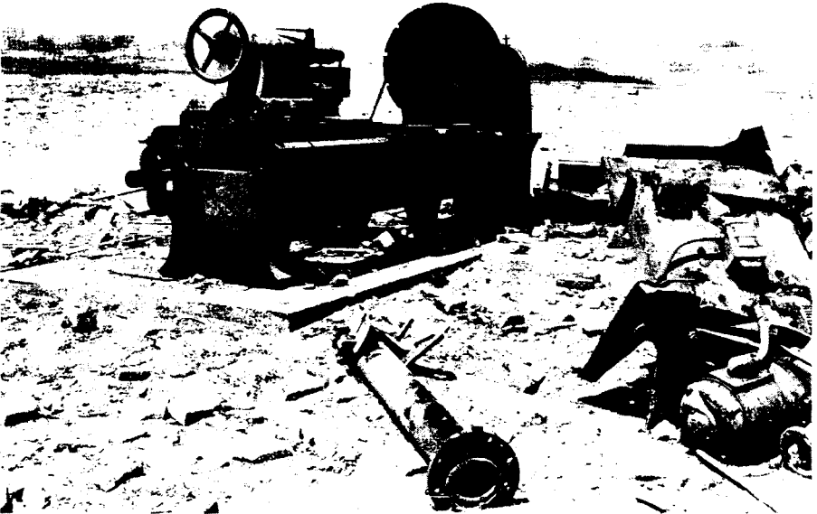
Figure 5.129b. Heavy-duty lathe after a nuclear explosion (10 psi peak overpressure).
