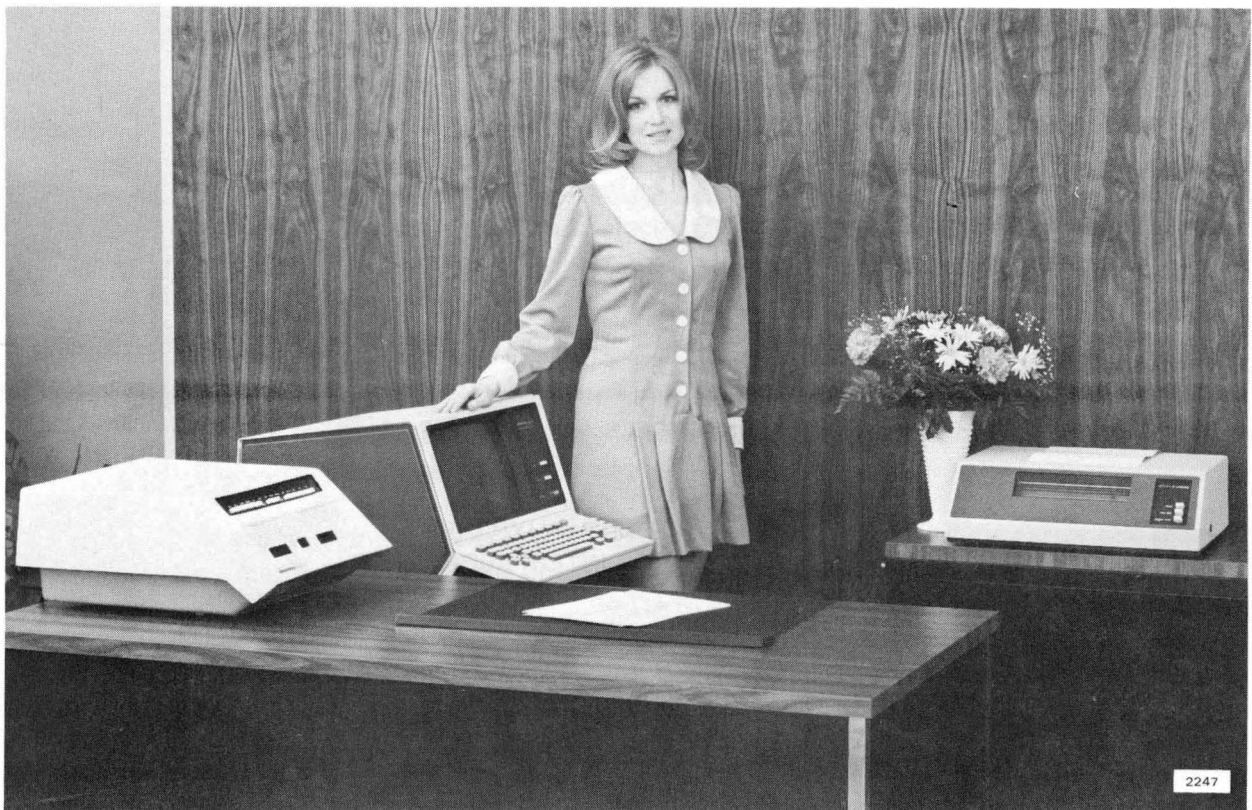
Figure 10. UNISCOPE 200 Terminal with Model 610 Tape Cassette System (left) and Model 800 Terminal Printer (right)
