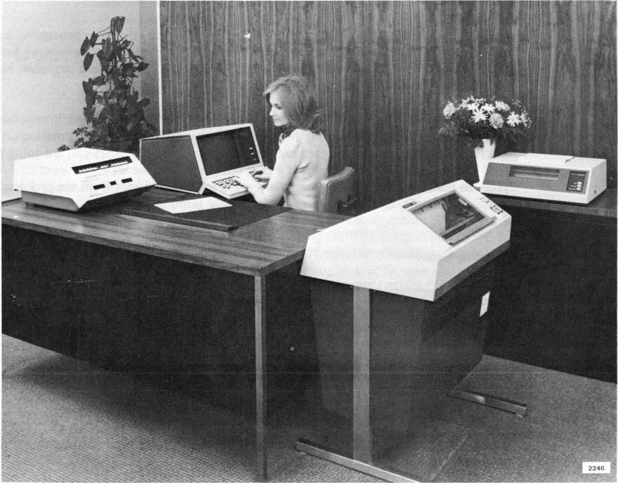
Figure 2. UNISCOPE 200 Display Terminal with Auxiliary Devices: Model 610 Tape Cassette System (left), Model 800 Terminal Printer (right rear), and Communications Output Printer (right front)
